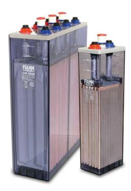
FIAMM's **LM** battery range can be used in standby mode or for duties requiring repeated charging and discharging operations (cycling applications). The **LM** battery range is specially designed for difficult environments and special applications such as solar and long discharge rates. Its tubular positive plates, a high reliability post seal and fully insulated connections among cells guarantee a long life even in the worst operating conditions.
